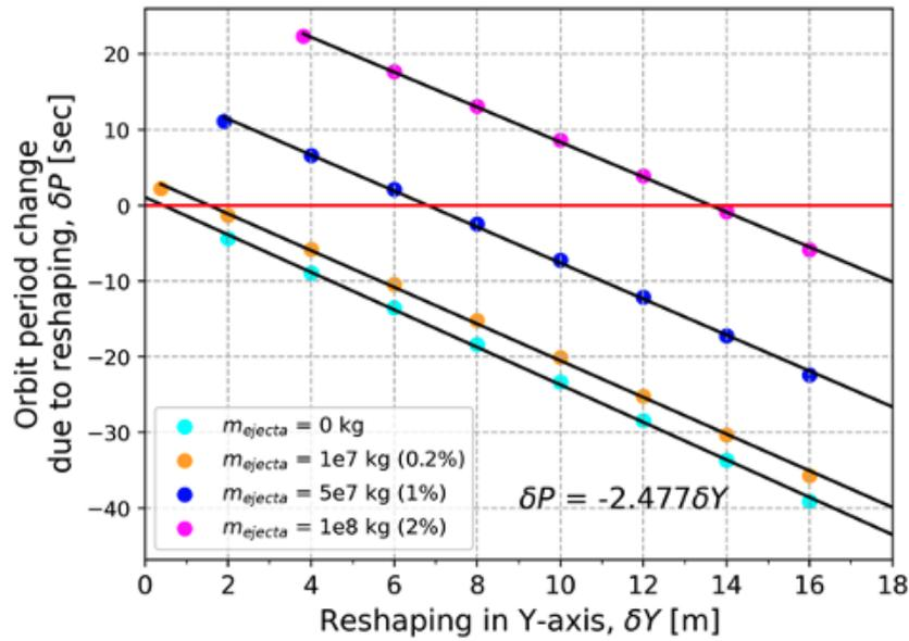
Figure 1. Orbit period change due to reshaping,  $\delta P$ , vs. reshaping in Y-axis,  $\delta Y$ . The data points in different colors show different  $m_{\text{ejecta}}$ . The black solid lines are linear fits to the data points.  $\delta P$  indicates the orbit period change relative to the nominal pre-impact orbit period (i.e., 11.92 h [10]).  $m_{\text{ejecta}} < 10^7$  kg cases are not shown as they are almost indistinguishable from the  $m_{\text{ejecta}} = 0$  kg case.
