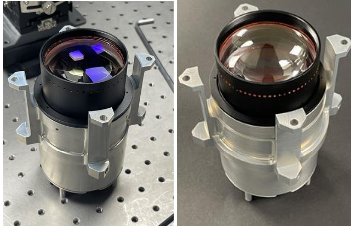
Figure 7. Assembled optical subsystems. (Left) VIS channel. (Right) UV channel.
