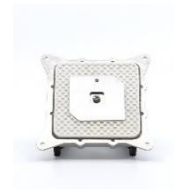
Figure 25. GNSS L1/E1 band antenna
