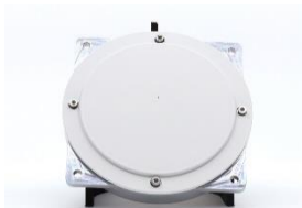
Figure 22. S-band TT&C antenna
