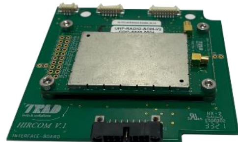
Figure 13. HIRCOM© UHF Transceiver for Cubesat
