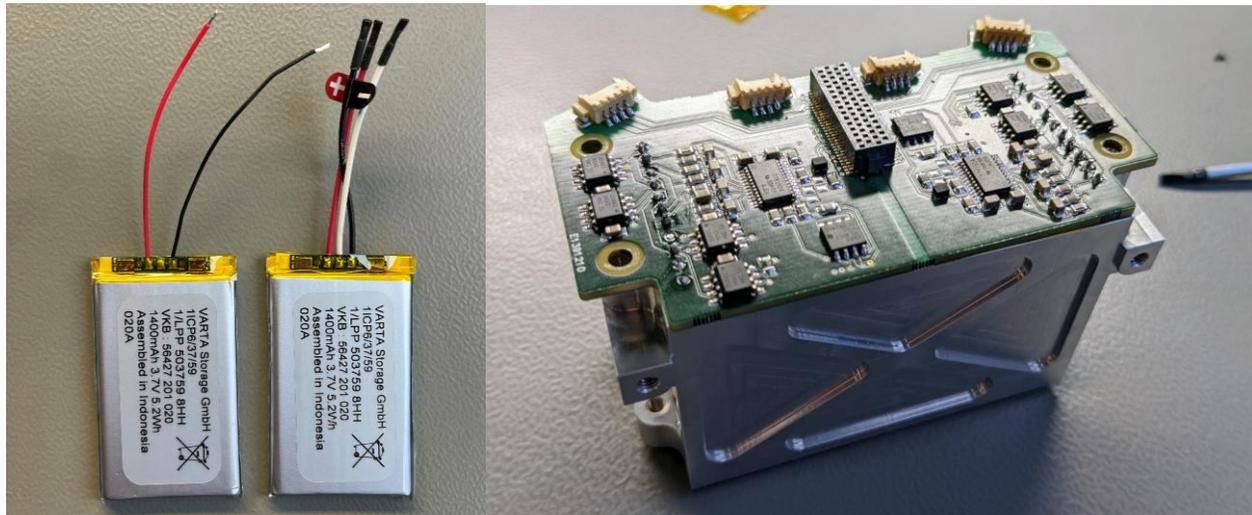
Figure 9: Battery cells and integrated battery compartment
