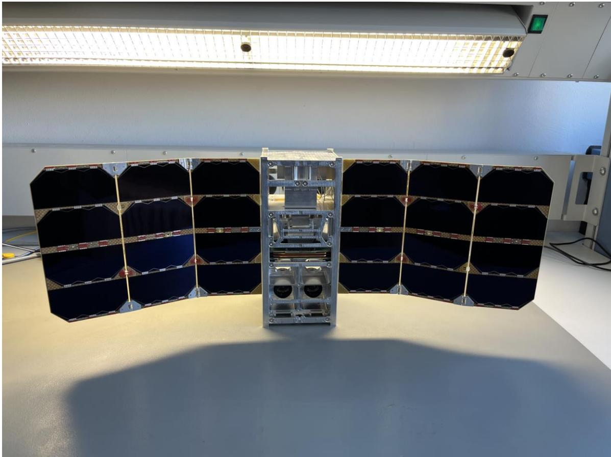
*Figure 8: Satellite model with deployed solar panels*
