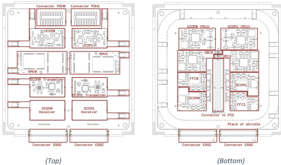
Figure 6: Multifunctional printed circuit board
