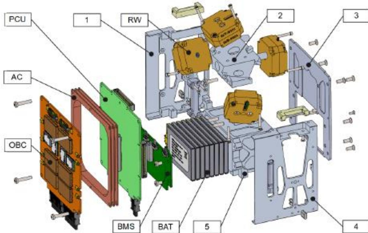
Figure 4: Explosion view of satellite bus
