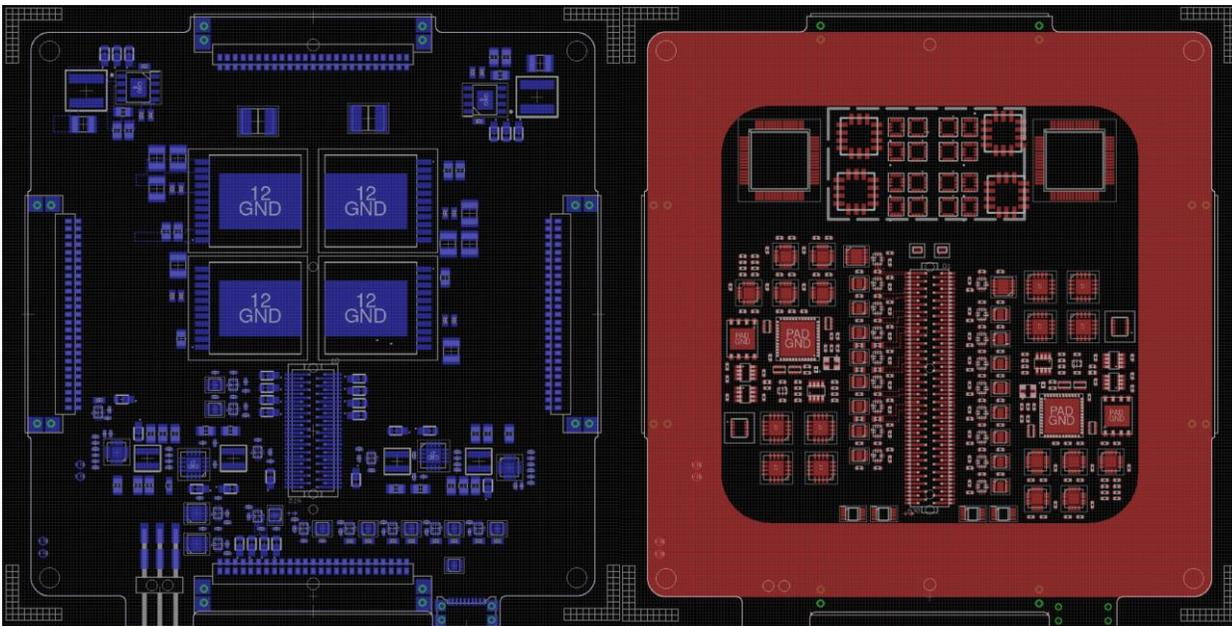
Figure 7: PCU and AOCS board
