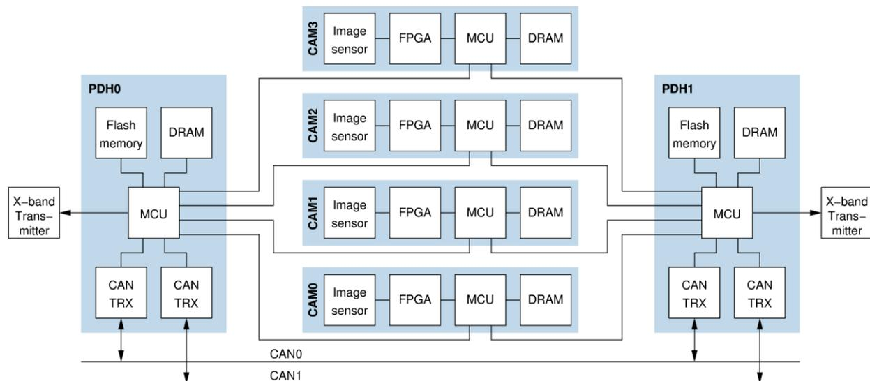
Figure 11: Block diagram of camera system and PDH
