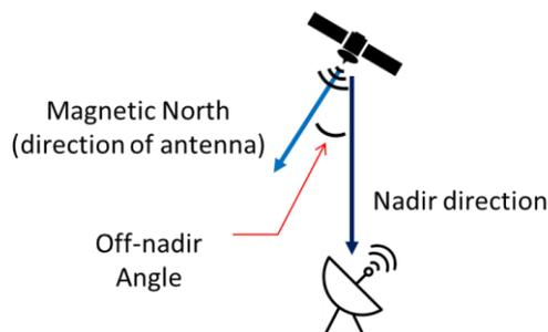
**Fig 3** Graphical definition of off-nadir angle.
