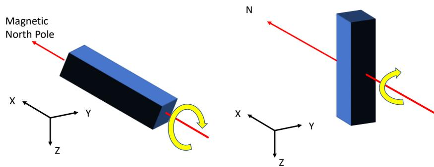
**Fig 1** Depiction showing free rotational axis for passive magnetic attitude control.
