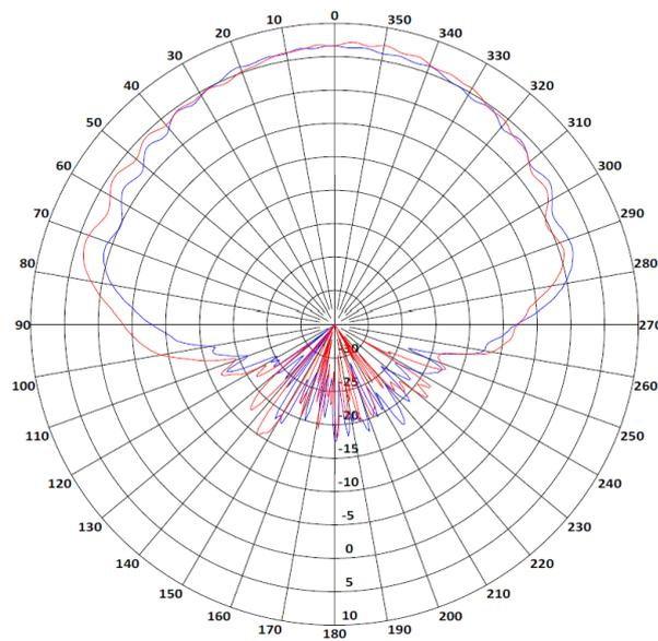
**Fig 5** Gain vs. angle plot of Haigh-Farr's X-band patch antenna at 8.25 GHz (credit: Haigh-Farr).
