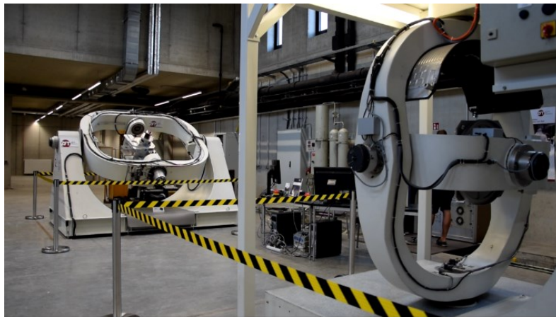
Figure 8. High precision, high dynamics turntables for testing relative attitude motion in a satellite formation to simulate inter-satellite links and joint camera observations
