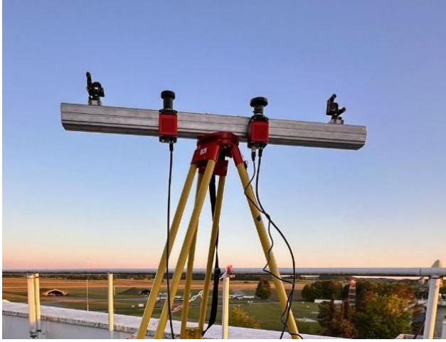
Fig. 5: Setup of the two near infrared InGaAs cameras with their fish-eye lenses, establishing the ASM hardware.
