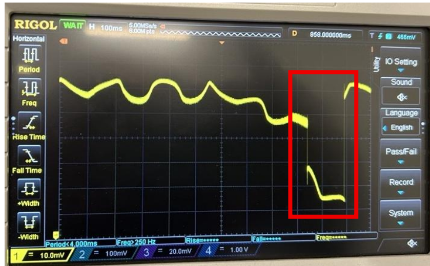
Figure 3. High power transmission spectrum, with the soliton step highlighted with the red box.
