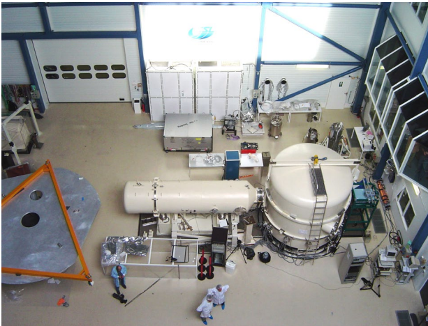
Figure 5. Focal-3 TVAC chamber at CSL. The left image shows an earlier TVAC configuration, but clearly showing the appendix used for the geometric collimator. The right image shows the current TVAC setup.
