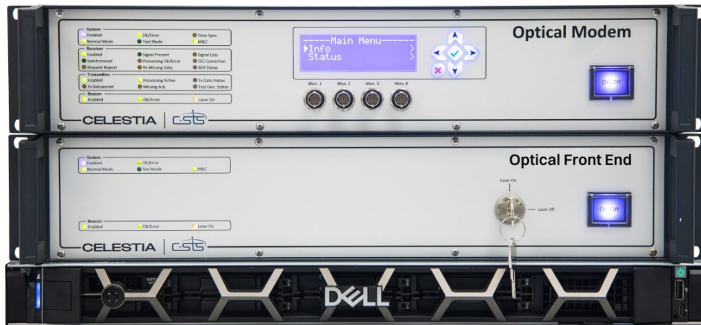
Figure 2-9 Picture of the Classical Optical Modem. Optical Modem unit containing the downlink modem opto-electronics, and the Optical Front End beacon unit containing the opto-electronics needed for generation, modulation and control of the uplink communication stream.
