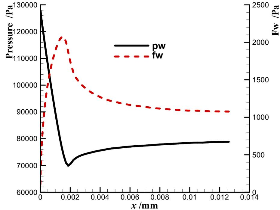
The pressure and wall friction distribution along the x-axis
