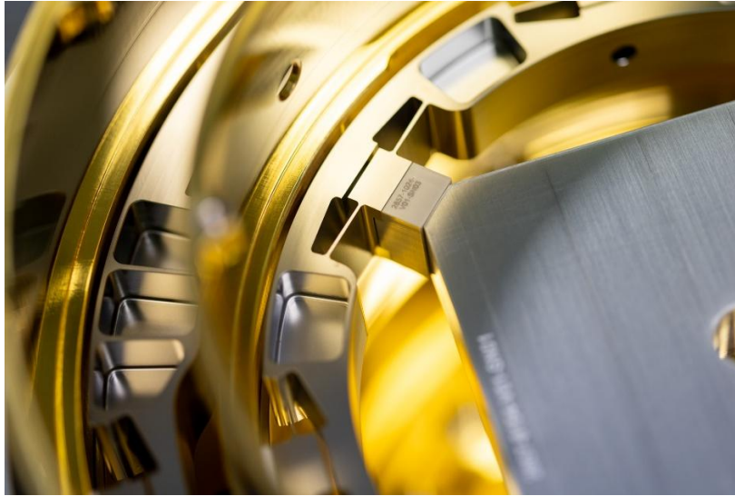
Figure 2: Blade and PEEK pad for conductive decoupling of the different thermal shielding layers. Picture was taken during the system blank assembly. Part on the right is a dummy part mimicking the cavity interface.
