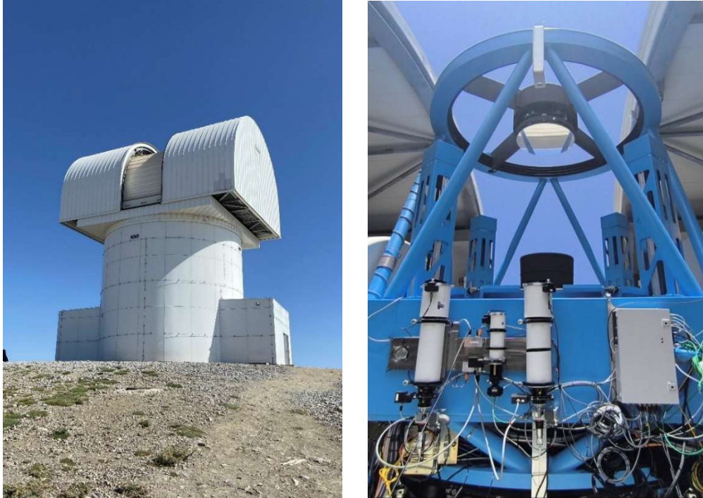
Figure 8. Helmos observatory (left) and two transmit and (in between) one receive module attached to the telescope (right).
