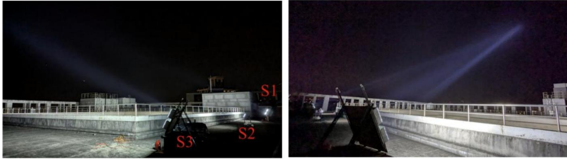
Figure 4. Nighttime operational deployment of the Active Ground Light Projection Method, illustrating the three strategically positioned wide-angle light sources (S1, S2, and S3) projecting calibrated beams toward the target satellite.
