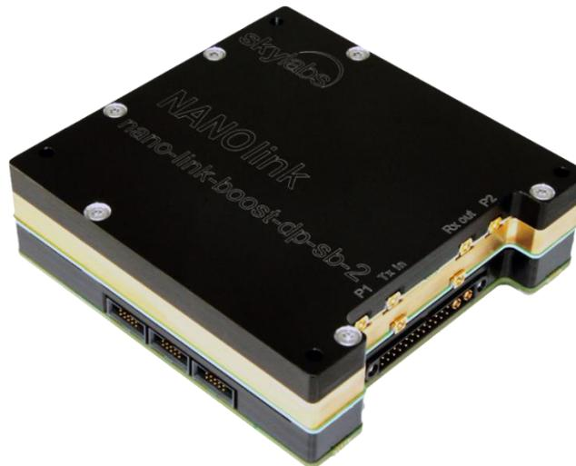
Figure 5: NANOlink-boost-dp High-throughput RF Transceiver Subsystem
