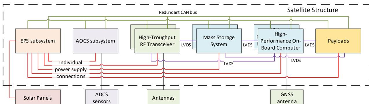
Figure 2: Modular satellite platform for Space Cloud Satellites
