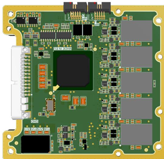
Figure 4: Mass memory subsystem
