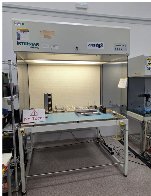
Figure 14. ISO 5 laminar-flow cabinet located within an ISO 8 cleanroom.
