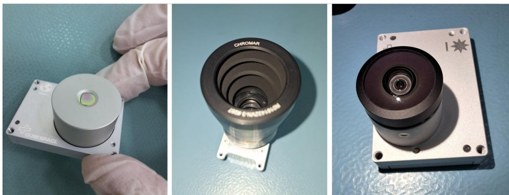
Figure 9. Left: Earth Horizon Sensor. Center: Star Tracker. Right: Fine Solar Sensor.
