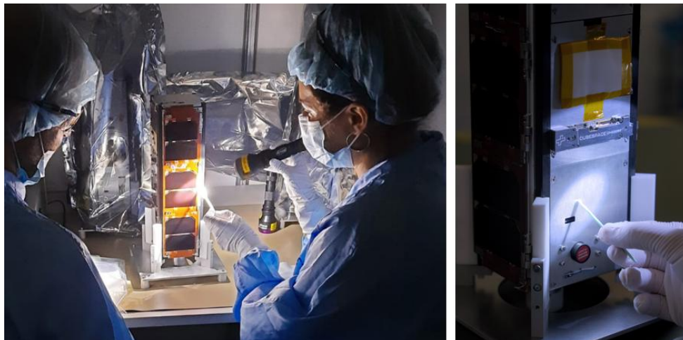
Figure 18. Visual inspections using white-light lamp during ANSER-WQ AIT campaign
