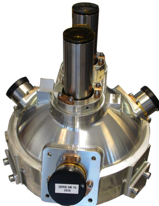
Figure 2: OSC Cupola with three STR CHUs and two NAC VBS CHUs.
