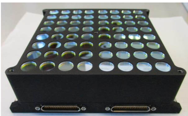
Figure 3: Double AMU in Flight Configuration. Primary and redundant side in single mechanical structure.
