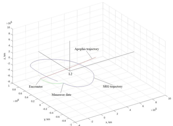
Figure 2. Transfer trajectory of the SRG space observatory to a close approach to Apophis
