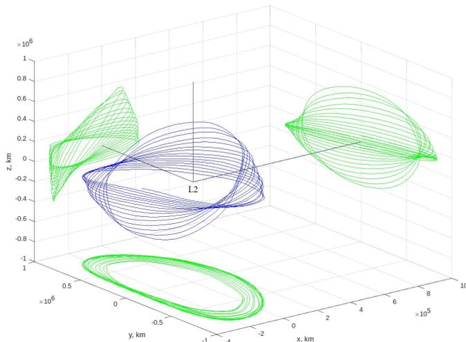
Figure 1. Trajectory of the SRG space observatory
