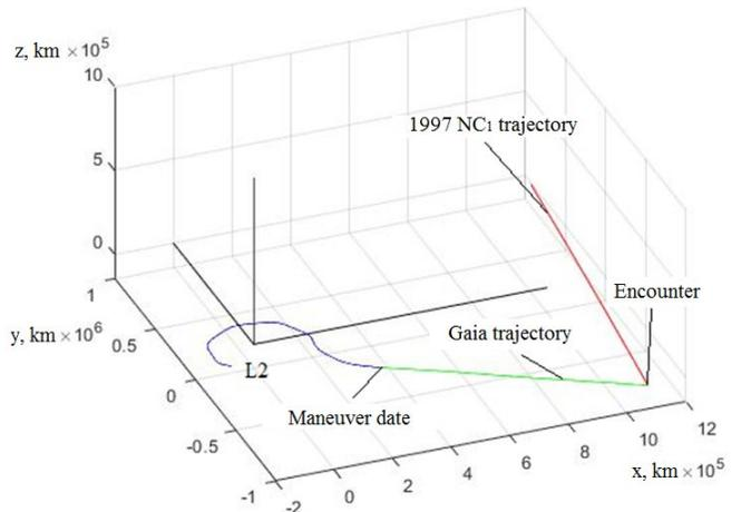
Figure 6. Transfer trajectory of the Gaia spacecraft to a close approach to the asteroid 1997 NC<sub>1</sub>
