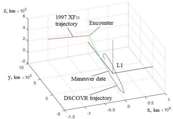
Figure 5. Transfer trajectory of the DISCOVER satellite to a close approach to the asteroid 1997 XF<sub>11</sub>
