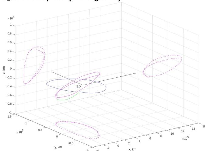
Figure 3. The trajectory of the SRG space observatory after the close approach to Apophis
