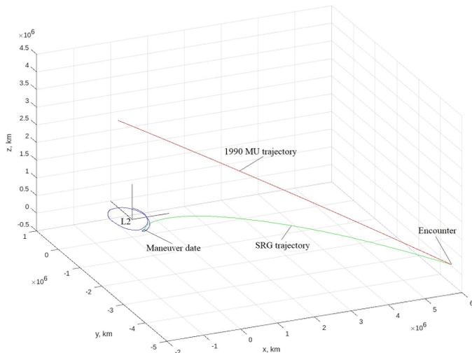
Figure 4. Transfer trajectory of the SRG space observatory to a close approach to the asteroid 1990 MU
