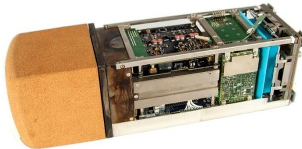
Figure 3: QARMAN prototype, showing the front P50 TPS (left).
