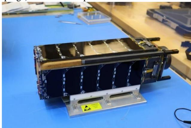
Figure 4: QARMAN flight model in stowed configuration.
