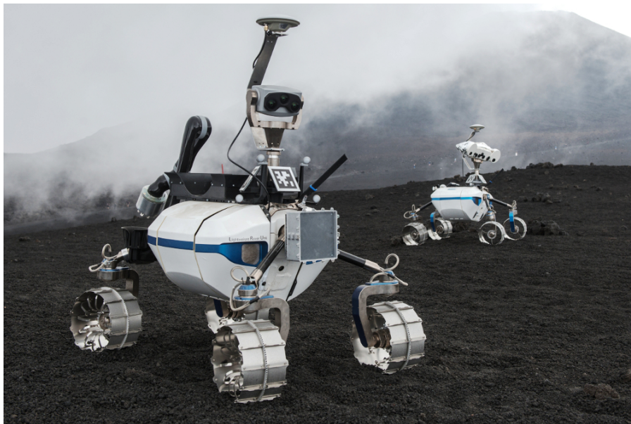
Figure 1: LRU1 and LRU2 on Mt. Etna, 2016. LRU2 features a robotic arm (front), LRU1 is equipped with additional scientific cameras (back).
