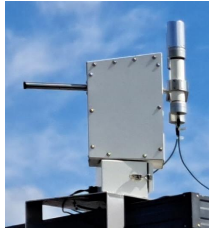
Figure 12 C-Dimm with Alt-Azimuth Mount at OGS-NZ
