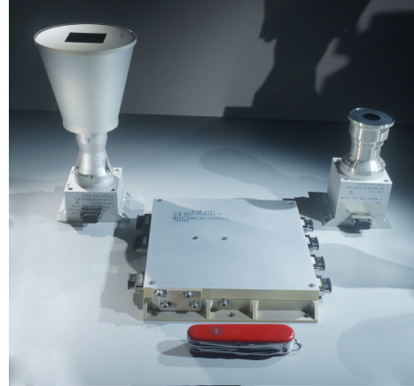
Figure 3: A Malin Space Science Systems ECAM-M50 (Monochrome) with NFOV (Narrow Field of View) lens (left), ECAM-IR3 (right), and ECAM-DVR4 (center). JCam will appear similar to this shown flight camera system with different lenses. Pocket knife for scale. Credit Malin Space Science Systems.
