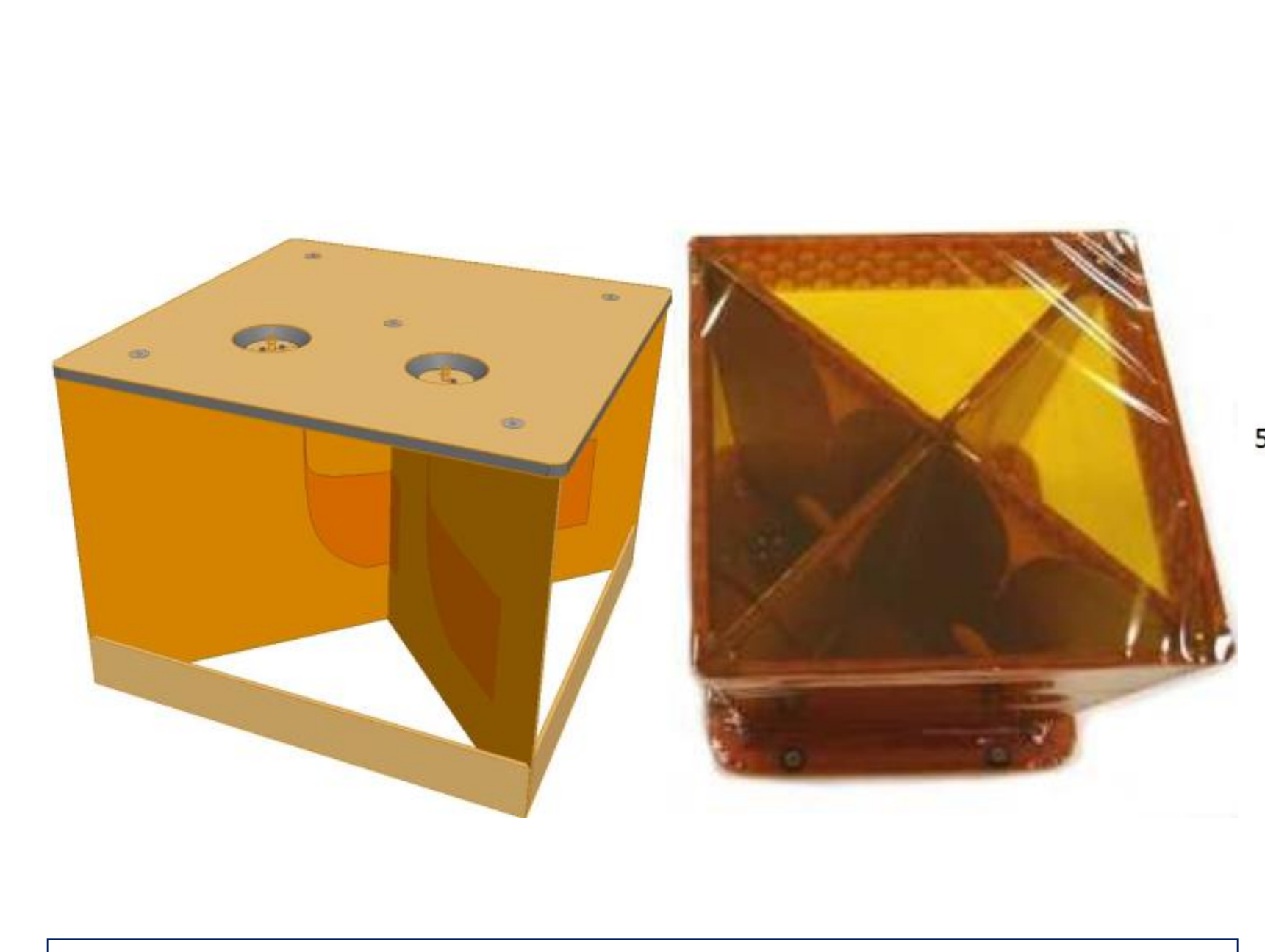
HFR ultra-broadband dual-polarized antenna ↑ 3D model – lightweight plate frame design – prototype ↑
