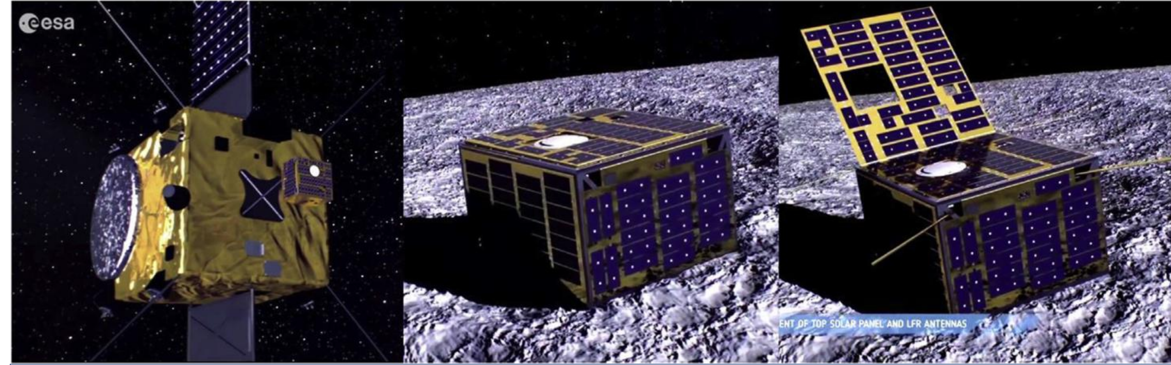
just separated from AIM – landed, self-righted, ready to relocate – opening the solar panel and extending antennae at operating site
