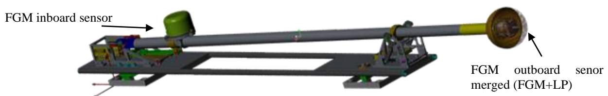
Figure 9 FGM-A boom. On the tip the merged sensor (fluxgate and LP)
