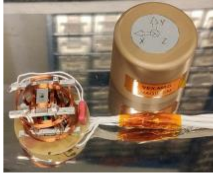
Figure 14 One fluxgate magnetometer sensor on the left, with its harness, and its cover on the right
