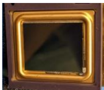
Figure 8 Lynred thermal detector after removing of protective window and FPI prototype
