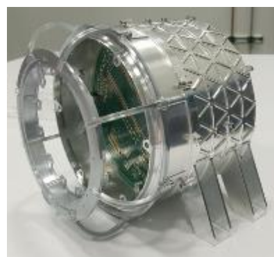
Figure 11 on the left schematic view of LEES, on the right prototype of LEES instrument
