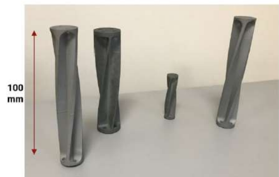
Figure 12: 4D printed rotary actuator
