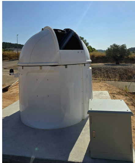
Figure 3. Optical ground segment deployed to conduct optical communications experiments with the 6GStar-Lab satellite.
