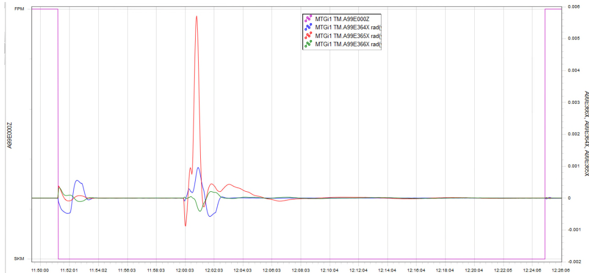
Figure 19. Attitude control error along the 3 sat axis during the EW manoeuvre (A99E364 = Z sat axis, A99E365 = Y sat axis, A99E366 = X sat axis)
