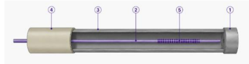
Figure 2. FBG temperature sensor layout 11 : (1) Tube lid; (2) Optical fibre; (3) Stainless-steel tube (4) protection tubing; (5) FBG sensor.
