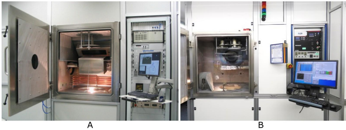
Figure 2. The IBS machines used for coating deposition. The machine in panel A uses a custom ion source, a classical rotating substrate holder, and can accommodate up to four different coating materials. This machine manufactured all three-material coating layer stacks for the use cases 1, 2, and 4. The machine presented in panel B features a 16 cm Veeco source, a planetary rotation, and can accommodate two coating materials. This machine manufactured two-material coating layer stacks for use case 3.
