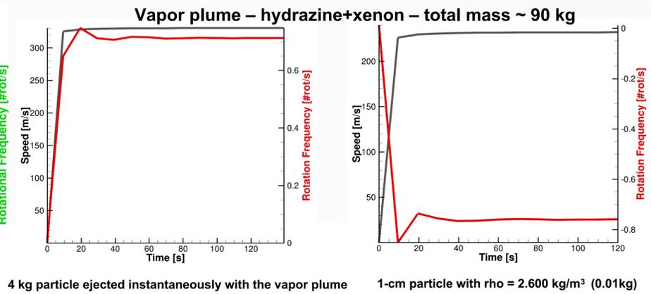
Particle velocity and rotation frequency for 50 velocity averaged velocities bins – velocities from 0.1 to 10 m/s. In all velocity bins we took the averaged velocity taking into account the velocity distributions and mass distribution within the bins at 150s by the impact simulations. Results show no influence on the shape for chunks with mas of hundreds kg.
