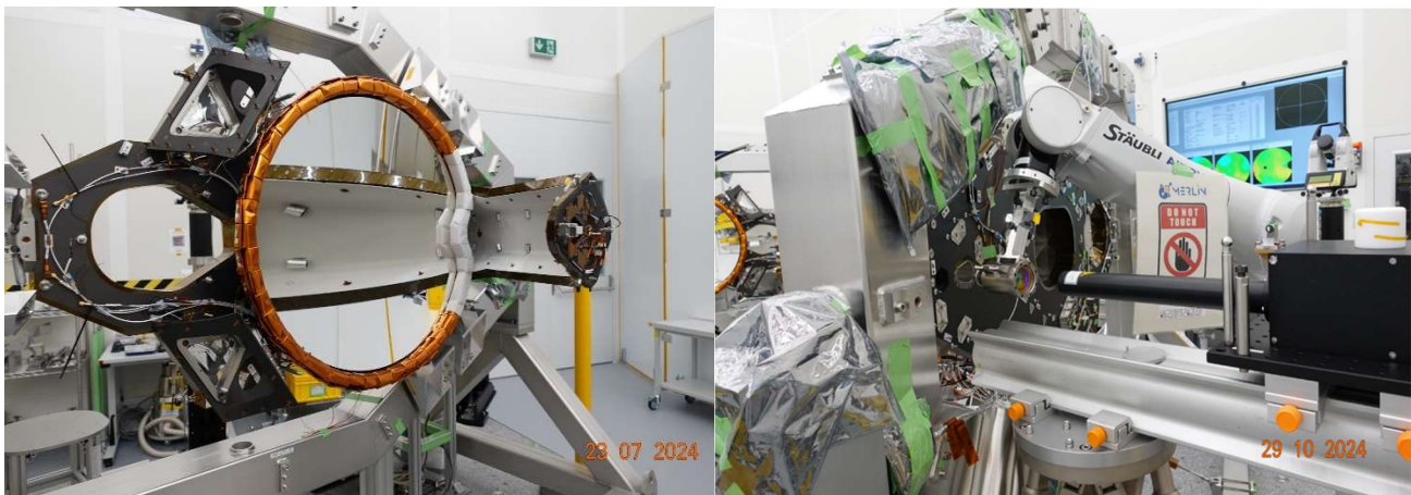
Figure 4-3: Merlin RX with integrated structure and M2 mirror (left) and with OCL in unfolded test configuration (right)
