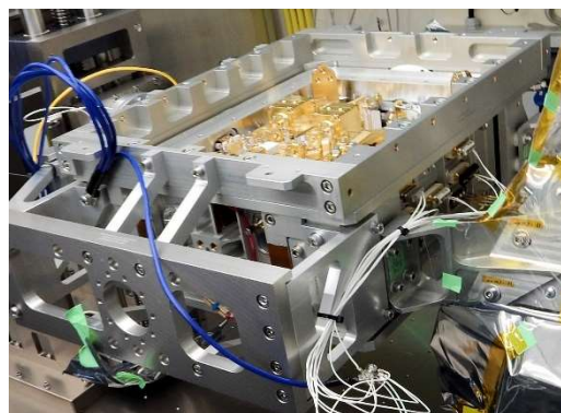
Figure 3-1: Laser (LAS): Laser housing (LASH) with integrated optical bench (LASO).
