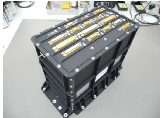
Figure 3-4: Merlin instrument control unit ICU – PFM
