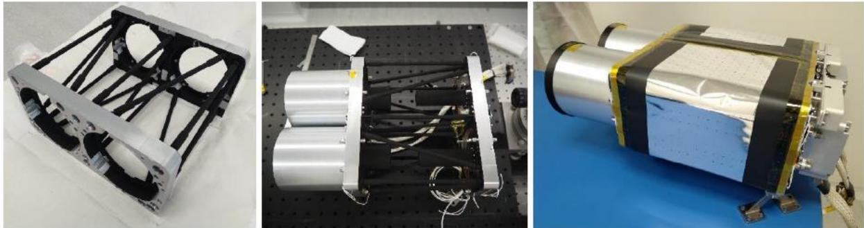
Figure 4. iSIM-90 VNIR camera for CASPR mission during integration at SATLANTIS
