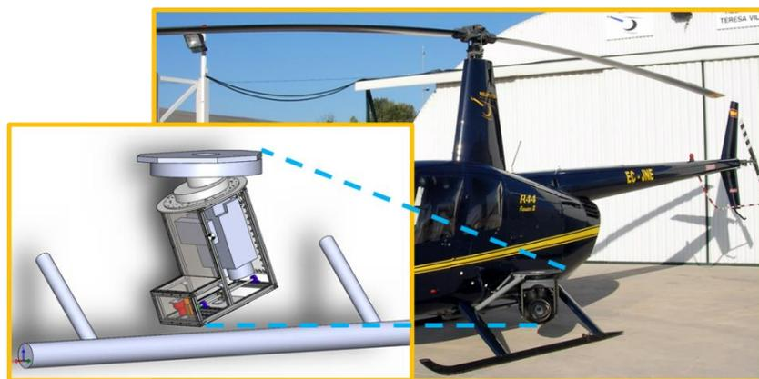
Figure 14. PM setup in a helicopter
