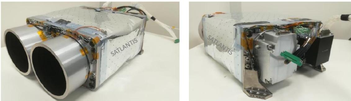
Figure 3. PM (Plane Model) fully integrated design of the opto-mechanics of iSIM-90 SWIR. The FM (Flight Model) will be slightly different, as a different VNIR detector will be used.
