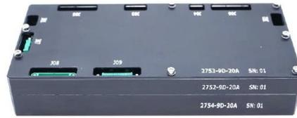
Figure 2. Electronic Control System box, with “SPoCK” electronic board (in charge of image acquisition and on-board image processing) and “Smart Heater” electronic board of the Thermal Control System (in charge of thermal stabilization) inside
