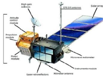
**Fig. 5: TOPEX/Poseidon satellite configuration (Credit CNES)**
