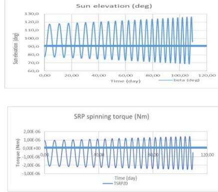
**Fig. 15: The sun elevation history generates an alternative profile for the SRP spinning torque with an uncertain mean value**
