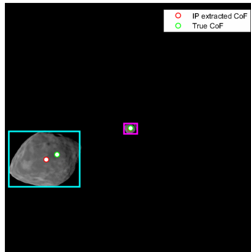
Figure 2: Far range navigation with true (green) and extracted (red) centre of figure (CoF).
