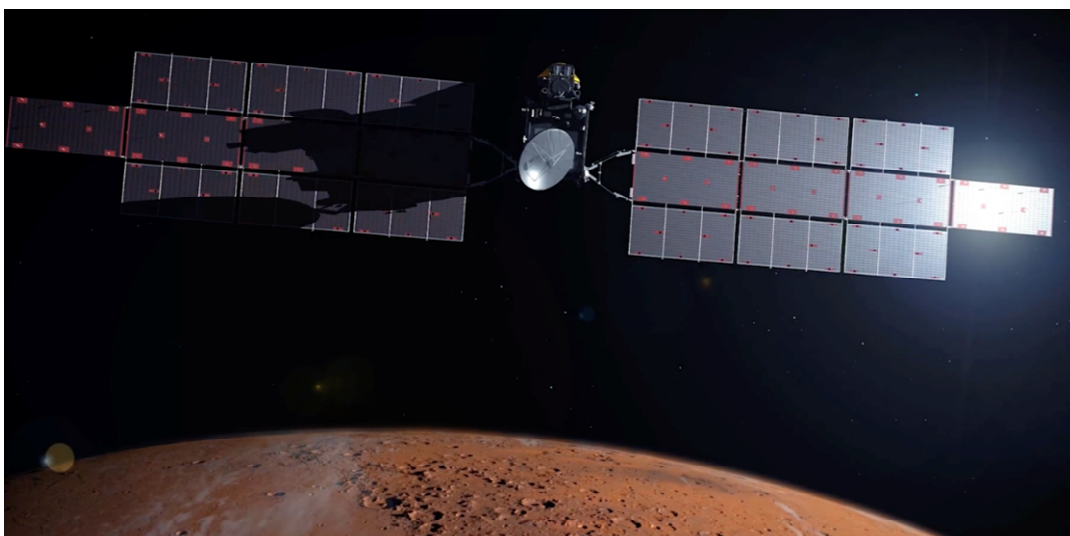
Figure 2. Earth Return Orbiter (ERO) with the Capture, Containment and Return System (CCRS) on its top. Credit: NASA/ESA/JPL-Caltech/GSFC/MSFC
