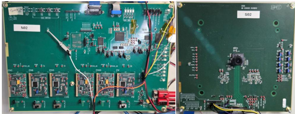
Figure 7. ASTERIA optoelectronic core 2D breadboard (left) with image sensor daughter board (right).
