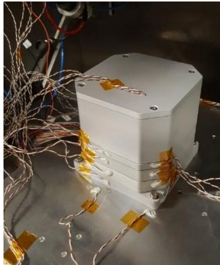
Figure 8: Astrix NS in the vacuum chamber for thermal tests
