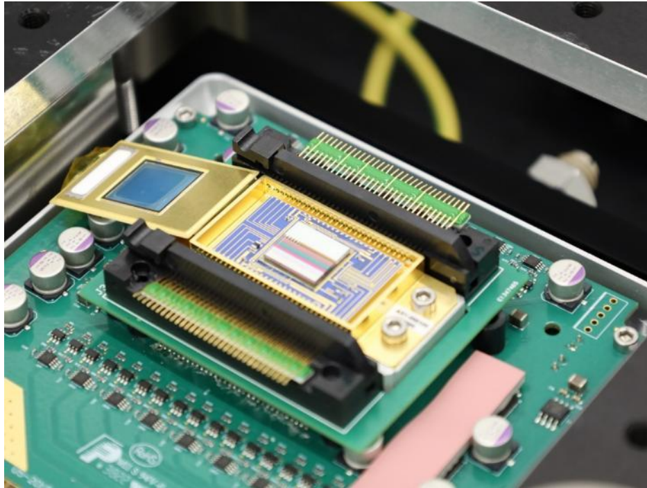
Figure 19: Detector with integrated filter, protection window opened
