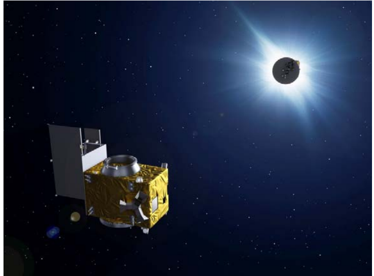
Figure 1, The PROBA3 formation flight Coronagraph. The distant Occulter spacecraft mask the sun disk, enabling the nearby Cronagraph spacecraft to study the corona. Source ESA
