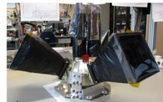
The OSC (Chaser) cupola with 3 STR cameras w baffles, and the two NAC center
