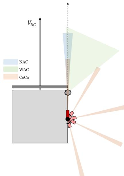
Figure 2: Rotating Mirror Assembly (RMA) allowing different orientations of the CoCa.
