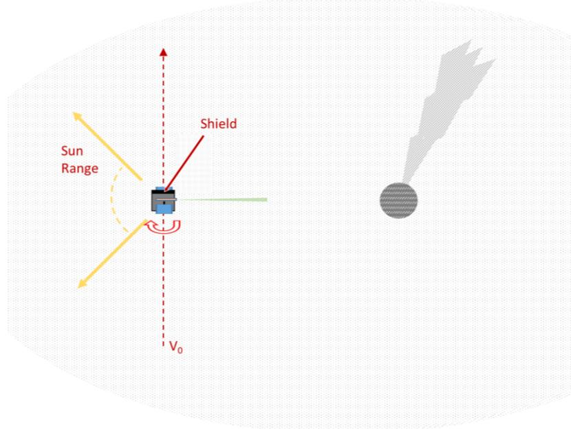
Figure 1: Encounter Strategy: the target maintains a fixed attitude to have only its ram face shielded – the SC can only rotate around its ram direction.
