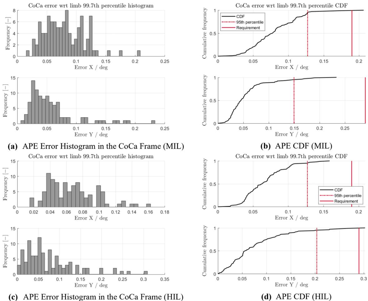
Figure 11: APE error in the CoCa frame and percentage of successful case over each step. A successful case is one that is within the threshold 99.7% of the time within a  $\pm 2h$  window.
