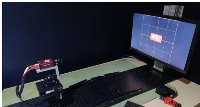
Figure 10: Optical Bench with the mounted camera and screen.
