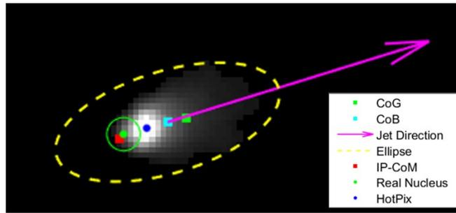
Figure 8: Jet Compensation Algorithm. In yellow the shape used to determine the jet's direction (in magenta) which is then used to determine the origin of the jet.
