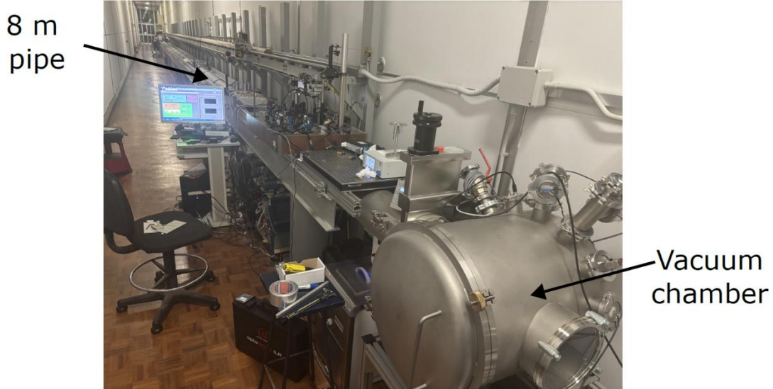
Figure 3. Overview of the experimental facility: the main vacuum chamber connected via the 8 m optical pipe to the secondary chamber.
