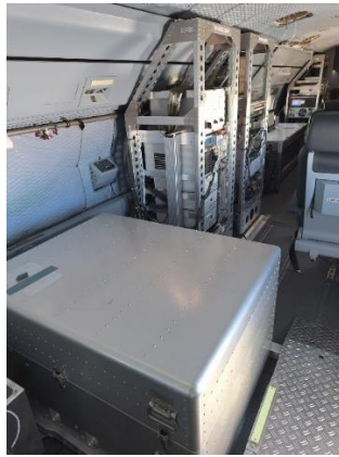
Figure 2. Photo of CHARM-F inside the German research aircraft HALO showing the optics box with the lidar transceiver in the foreground and its two electronics rack in the background.
