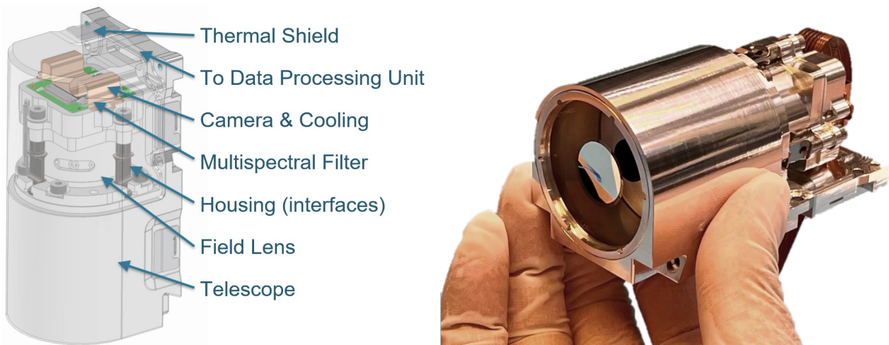
Figure 7. The TT-245-40 telescope & camera unit and its internal components. A single unit measures 50 \times 50 \times 100 mm, thus 2P units in the pocket qube standard. This fits perfectly as the main payload in a Alba Orbital Unicorn 2 platform. The mass is 384 grams.
