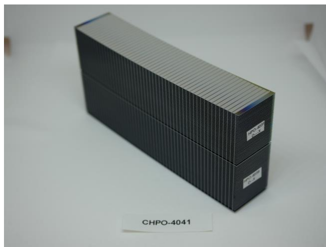
Figure 3: Example row-15 CHPO consisting of two bonded SPO stacks. Reproduced from the attached MM-development paper [4].
