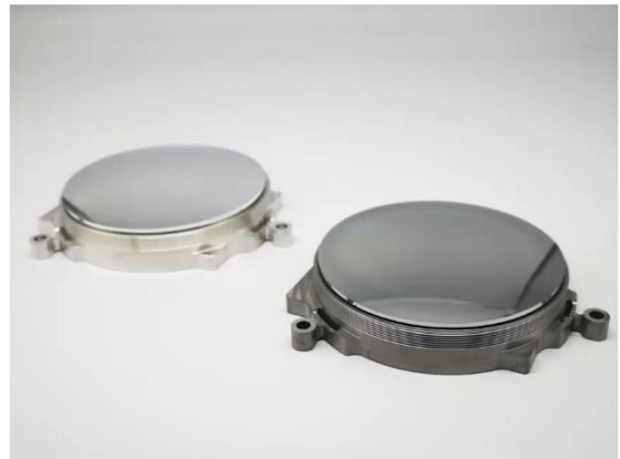
Figure 5-2: M2 mirror made of Al6061 (left) and AlSi40 (right) after SPDT.
