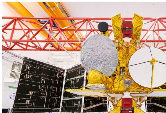
Figure 2. SWOT satellite during solar panels deployment tests at the Thales Alenia Space facility in Cannes, France. Credit: Thales Alenia Space.
