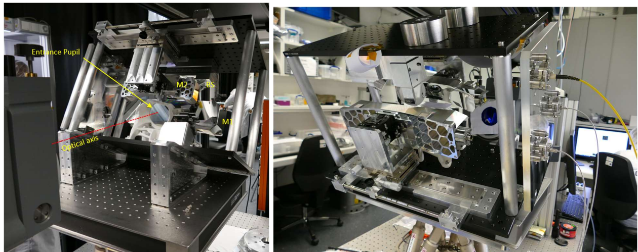
Figure 22. Left: Frontal view of the OSTEELoS breadboard during the WFE measurements at LoS 0°. Right: Back view with atto-cubes for mirrors M1 and M2.
