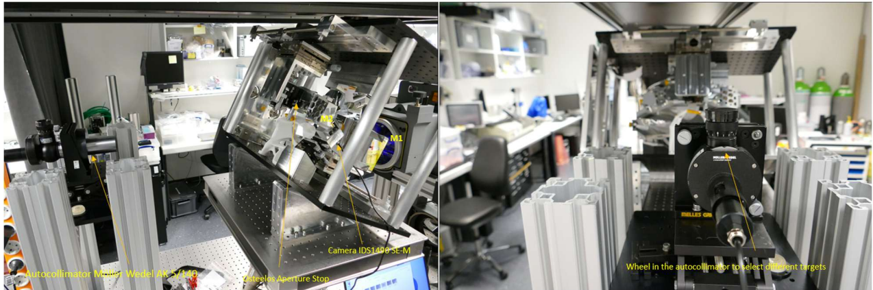
Figure 26. Alignment of the auxiliary camera with the autocollimator 5/140.
