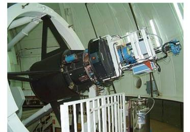
The Wide Field Camera installed on the 2.5m Isaac Newton Telescope
