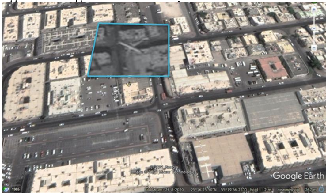
Figure 4-2. Downloaded geolocated image of an airborne aircraft detected in reference Maxar World View-3 multispectral imagery using SpaceCloud SaraniaSat application. The downloaded geo image has been overlaid on Google Earth.
