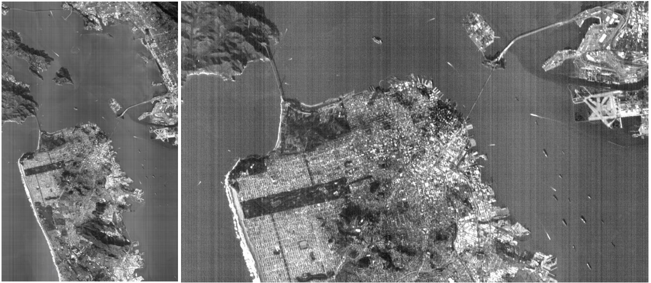
Figure 12. NAPA-2 RAW and unprocessed thumbnail (left) of San Francisco and a snippet of the full RAW unprocessed blue band showing ships and wakes and the shadow of the Golden Gate Bridge.
